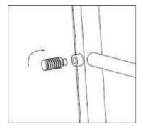
6. Align and push the rail brackets on the radiator onto the wall brackets secured to the wall. Secure the two together with the connecting screws provided (insert through the slot in the bracket) and tighten (be sure not to overtighten).
