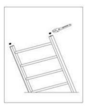
2. The rear of the towel rail has four location holes to fix the brackets. Measure the distance between all the location holes and mark these on the wall in the required location, use a spirit level to ensure these are horizontally and vertically aligned.
