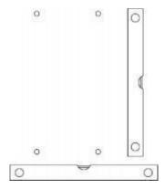
3. Using the drill and 8mm drill bit, drill into the marked positions then insert the wall plugs and tap flush to the finished wall surface.
